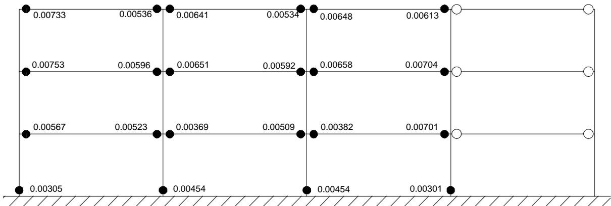
Figure 7. Peak Plastic Rotation Demands in Moment-Resisting Frame Under 1.495 Times El Centro
