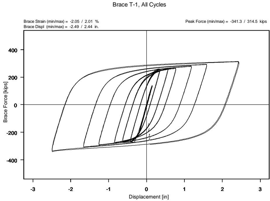
**Figure 11. Hysteretic Behavior of Brace Specimen T-1 in Basic Loading History Test**
