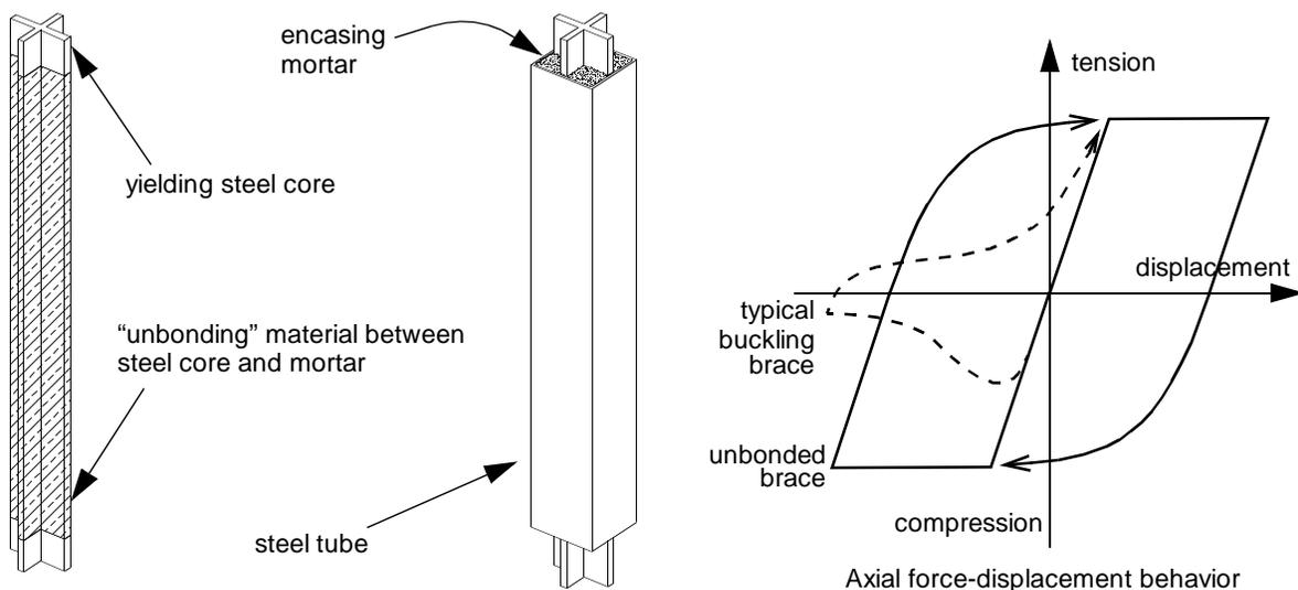
**Figure 1. Schematic of Mechanism of Buckling-Resistant Unbonded Braces**
