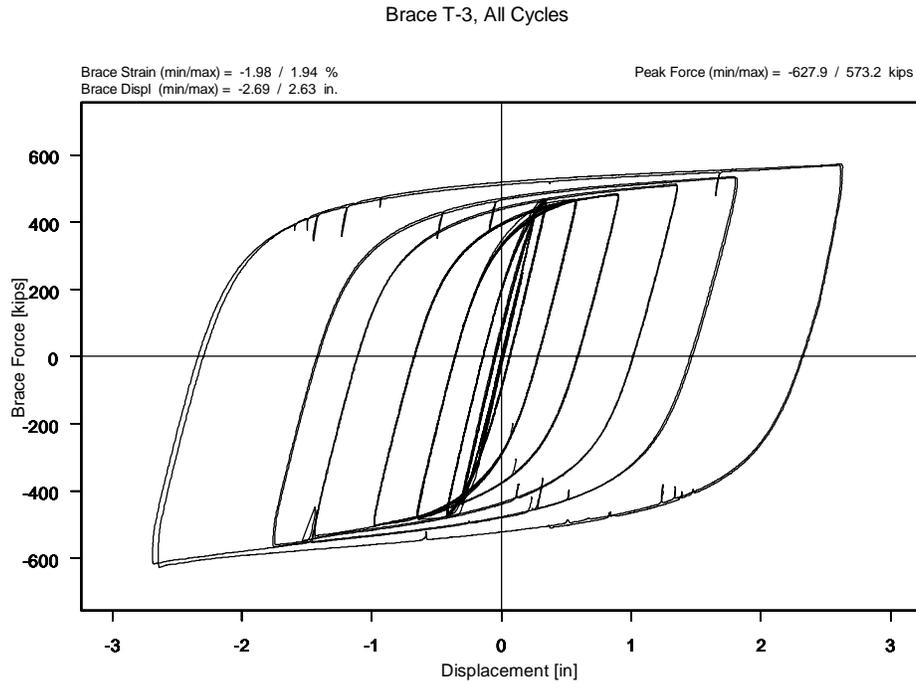
**Figure 13. Hysteretic Behavior of Brace Specimen T-3 in Basic Loading History Test**
