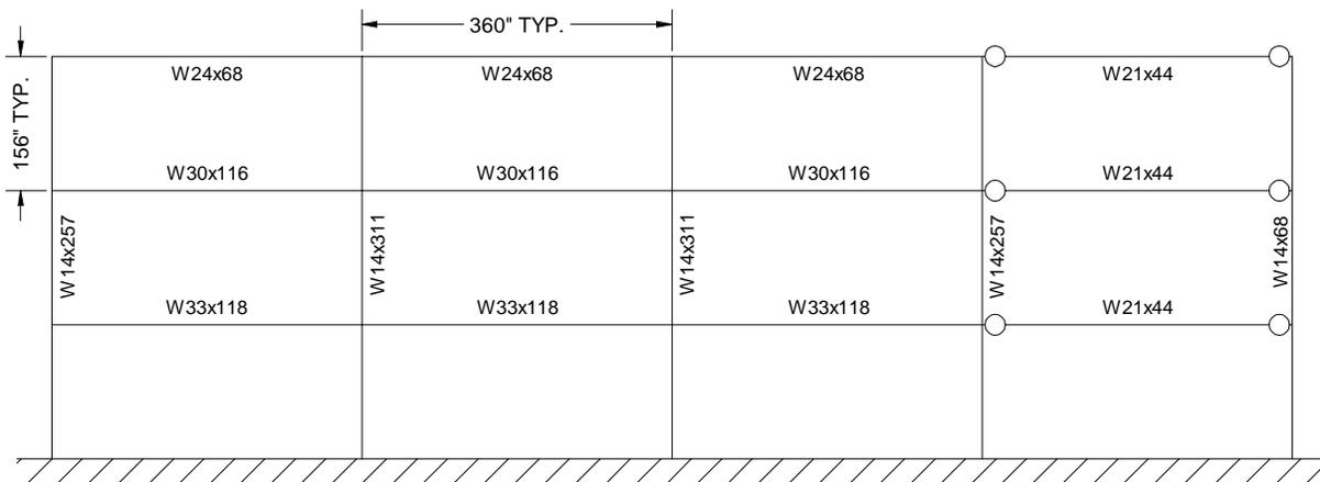
Figure 2. Three-Story Special Moment-Resisting Frame from FEMA/SAC Project
