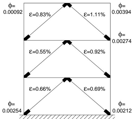
Figure 8. Peak Plastic Rotation Demands and Brace Strains in Unbonded Brace Frame Under 1.495 Times El Centro
