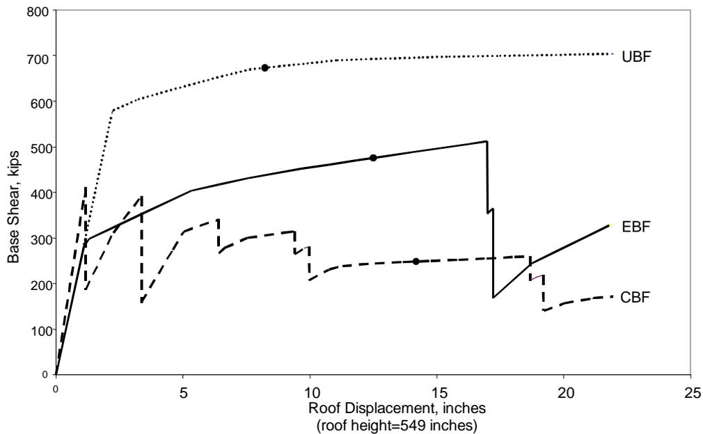
**Figure 18. Results from Pushover Analyses of Three Different Braced Frame Systems**
