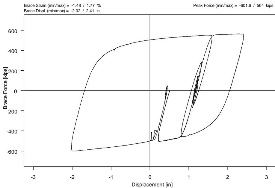
**Figure 16. Hysteretic Behavior of Brace Specimen T-3 During Sylmar Earthquake Test**
