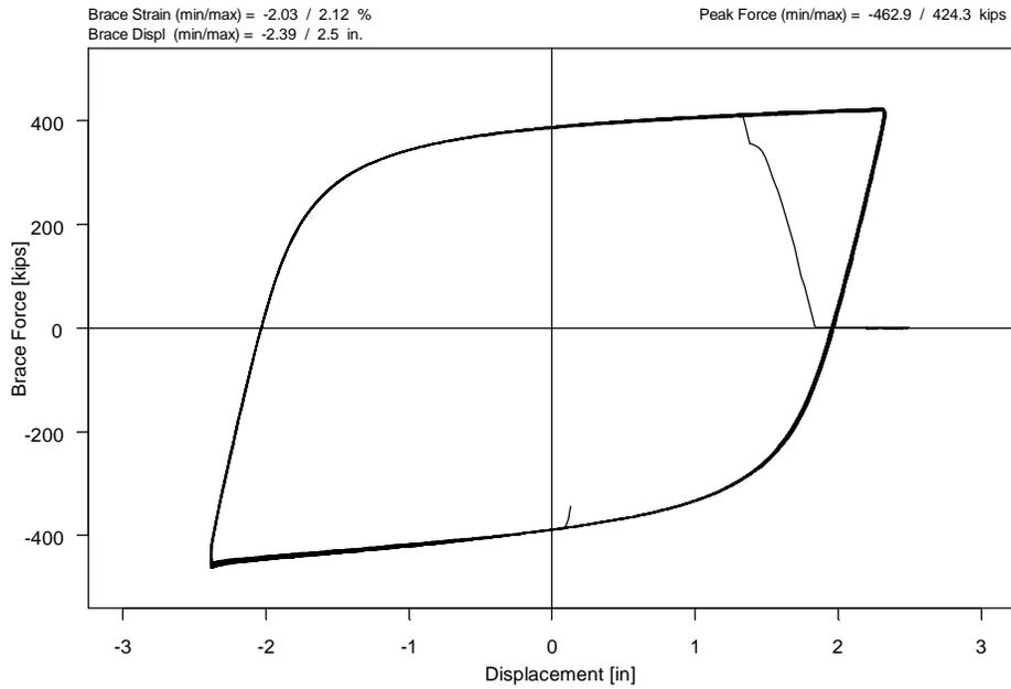
**Figure 15. Hysteretic Behavior of Brace Specimen T-2 During Low-Cycle Fatigue Test (15 complete cycles shown in the figure prior to failure)**
