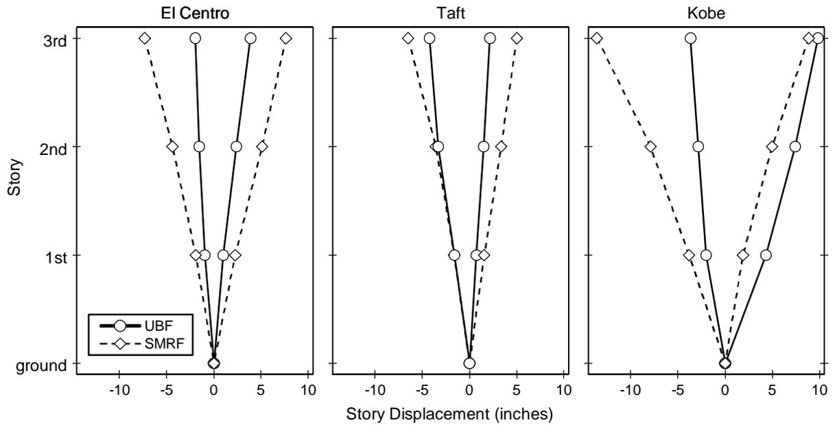
Figure 5. Story Drift Profiles for Unbonded Braced Frame and Moment-Resisting Frame
