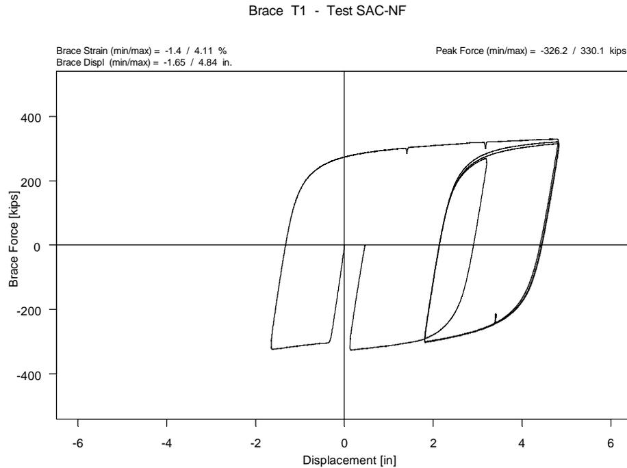
**Figure 14. Hysteretic Behavior of Brace Specimen T-1 in SAC Near-Field Loading Test**
