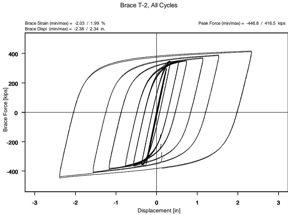
**Figure 12. Hysteretic Behavior of Brace Specimen T-2 in Basic Loading History Test**
