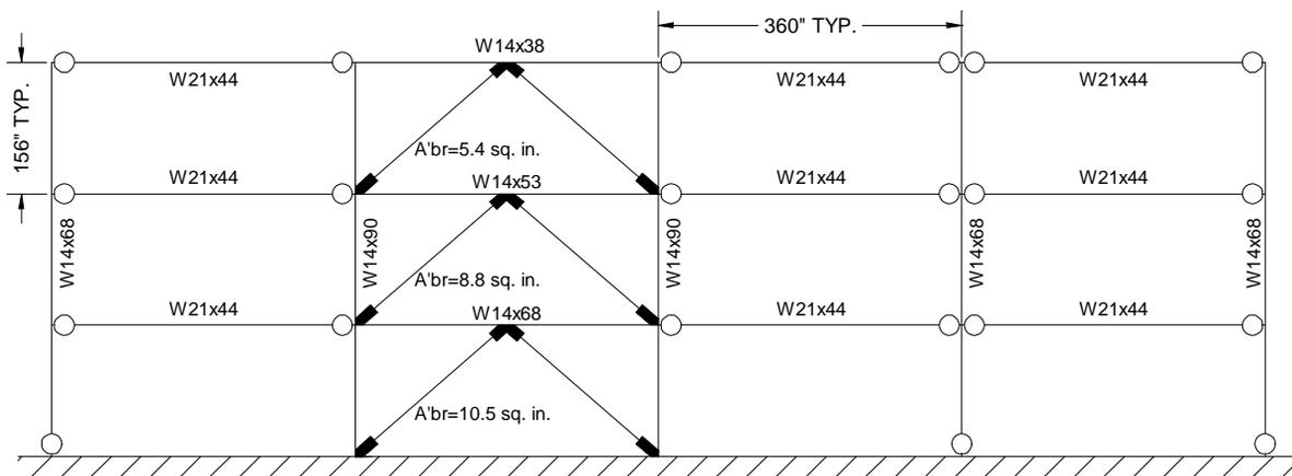
Figure 3. Three-Story Frame Redesigned with Unbonded Braces
