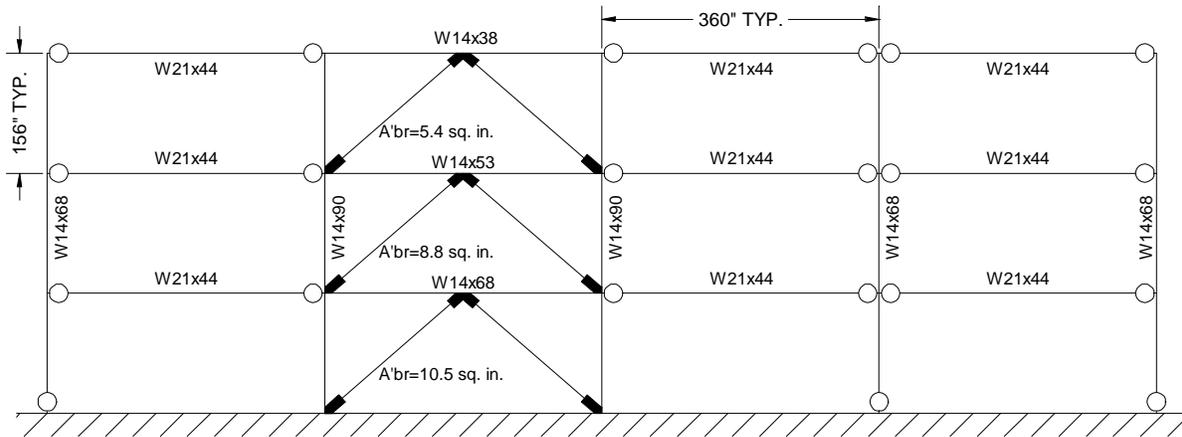
Figure 6. Three-Story Frame Redesigned with Unbonded Braces
