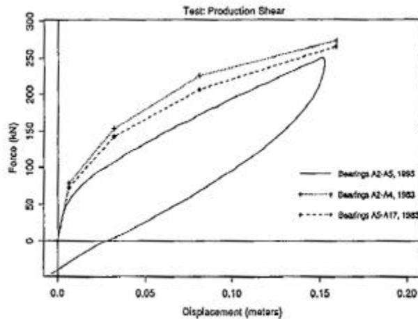
**Figure 1. Comparison of Original Force-Displacement Behavior (Derived from 1983 Tests) with that Recorded in 1995 Tests**
