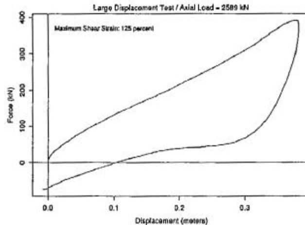
**Figure 2. Force-Displacement Behavior During Test to  $\pm 0.41$  m ( $\pm 16$  in.)**
