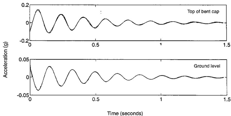
Fig. 2: Bent 4 free vibrations (exptal and analytical responses shown)
