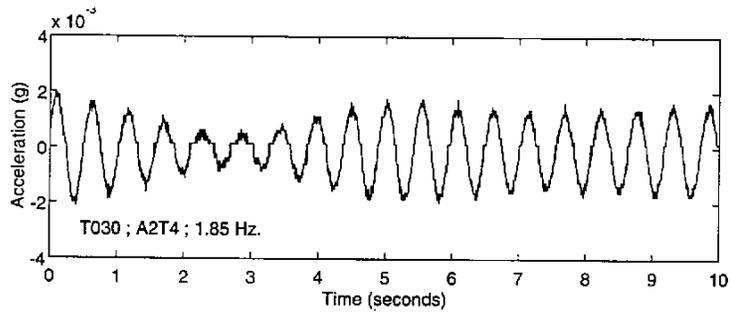
Fig. 4: Typical transverse forced-vibration response of isolated bridge, showing beating
