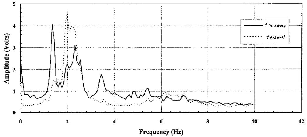
Fig. 9: Ambient Vibration response of completed isolated bridge - frequency domain
