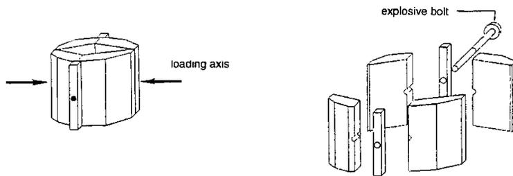
Fig. 5: Schematic of ISMES collapsible device
