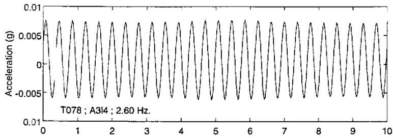
Fig. 3: Typical longitudinal forced-vibration response of isolated bridge
