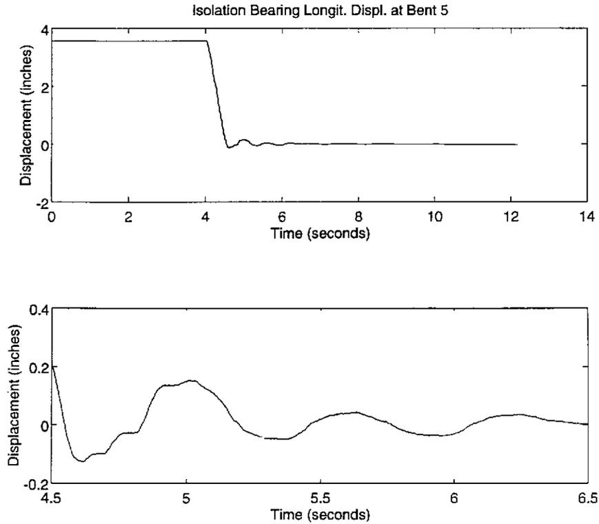
Fig. 8: Displacement time history for quick-release test no.3
