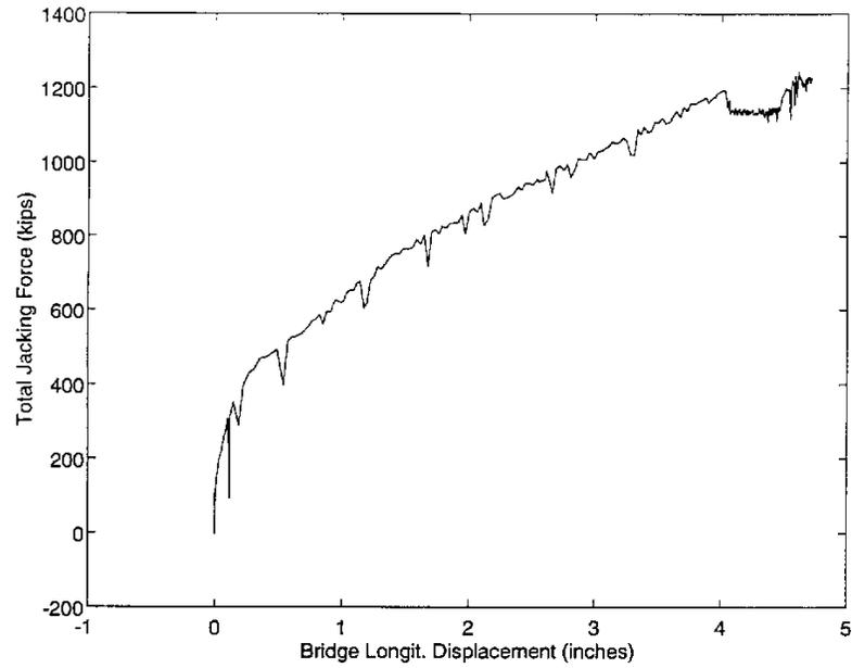
Fig. 7: Force-displacement plot for loading stage of quick-release test no. 2
